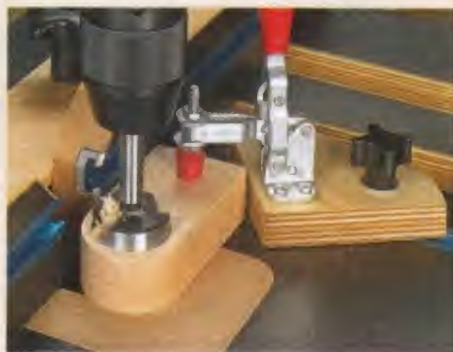
◀ Hold-down. A toggle clamp mounted to a small plywood base makes a handy hold-down for small workpieces.
