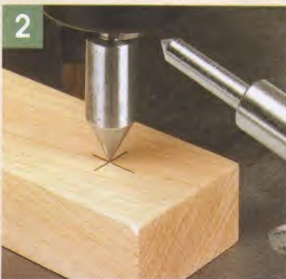
◀ To the Point. A machined pin makes it easy to locate the exact centerpoint for drilling a hole.
