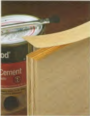
▲ Plain Edgebanding. Contact cement creates an "instant" bond for plain edgebanding.
