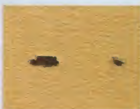
◀ Hole Size. The head on an 18-gauge brad leaves a big hole (left). But the hole from a 23-gauge pin is far less noticeable (right).
