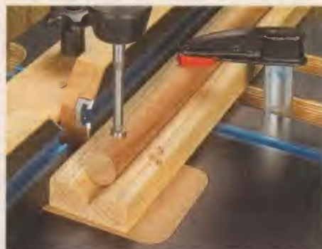
◀ Clamping Ease. Slots in the table make it easy to use bar clamps to securely hold the workpiece.
