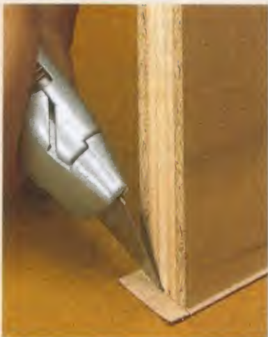
▲ Trim the End. A sharp utility knife makes quick work of trimming the end of the edging flush.
