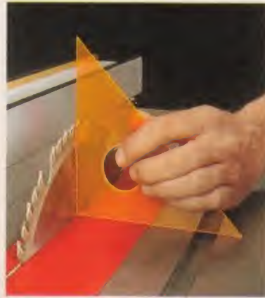
▲ Set the Blade to 90°. A drafting triangle makes it a snap to square the saw blade to the table.
