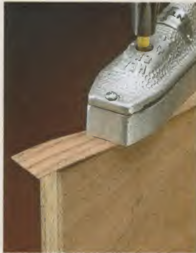
▲ Adhesive-Backed. Gluing this material in place is just a matter of melting the adhesive with an iron.
