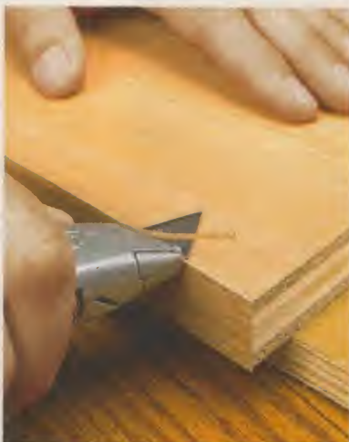
▲ Next, the Edge. To trim the edge flush, rest the blade against the face of the workpiece.
