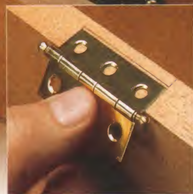
▲ Top-Notch Results. Clean up the corners with a chisel so the hinge slides perfectly in place.
