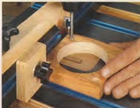
◀ Stop Block. Add a stop block to make drilling repetitive holes or mortises a simple, accurate task.
