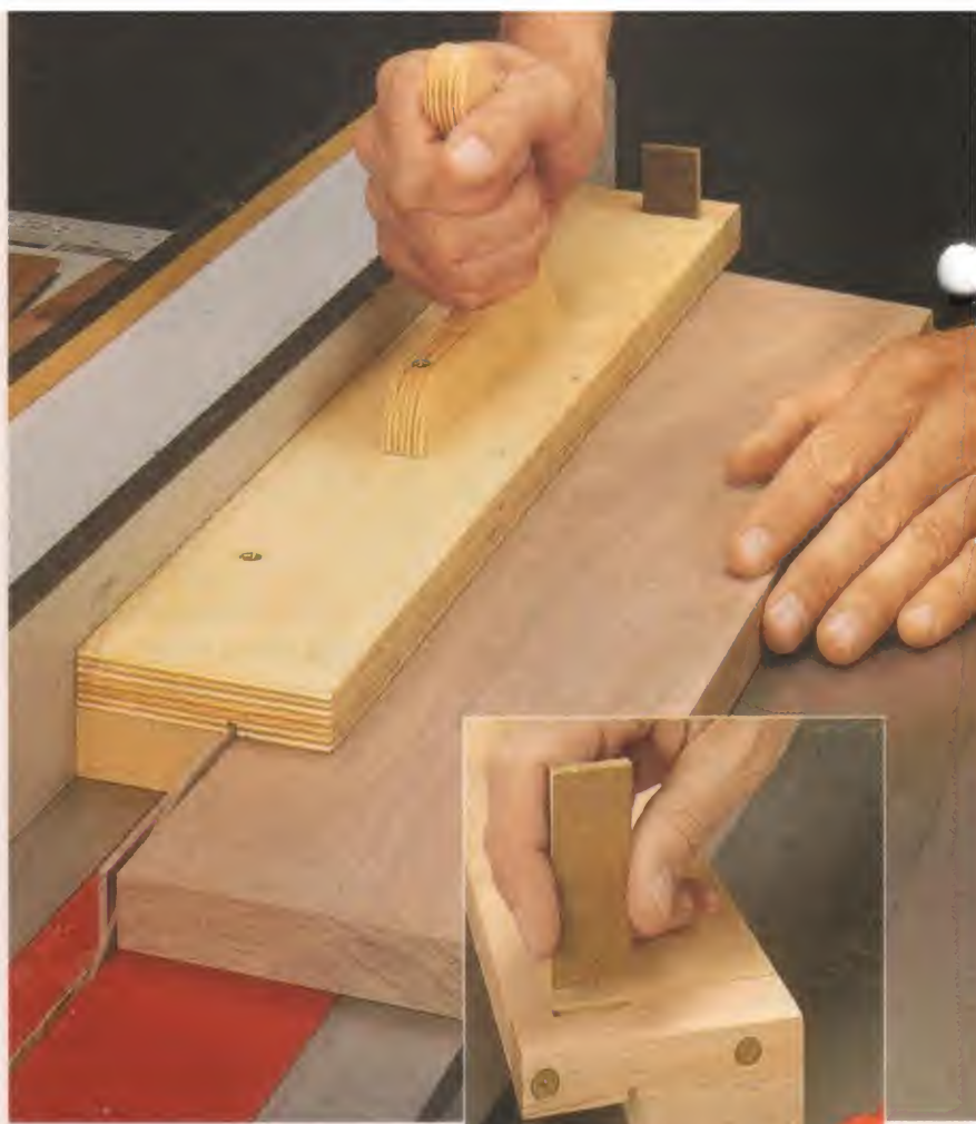
▲ Short Strip Jig. A replaceable stop (inset photo) pushes the workpiece through the blade when ripping short strips.
