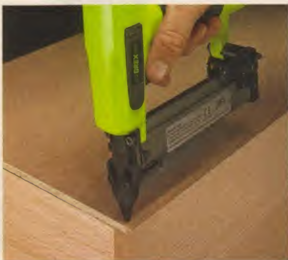
▲ No Clamps Needed. For small projects, like this small cabinet back, you can use pins as "clamps" to hold pieces in place while the glue dries.
