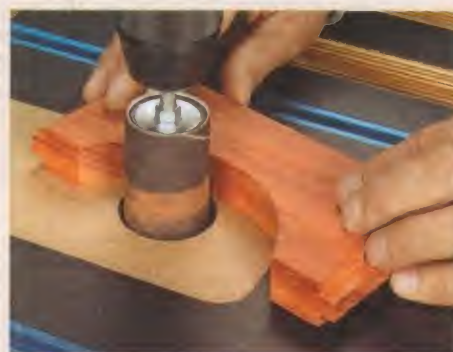
◀ Custom Inserts. Inserts can be made for specialized tasks like drum sanding. They help funnel dust and chips to the dust collection system.
