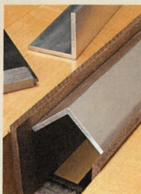
▲ Square Up Corners. To true up aluminum angle, tap the corner to spread the angle, or squeeze it in a vise if the angle is too wide.
