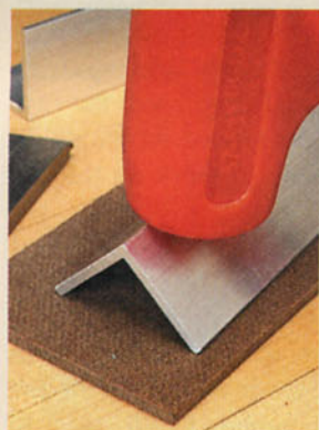
▲ Square Up Corners. To true up aluminum angle, tap the corner to spread the angle, or squeeze it in a vise if the angle is too wide.
