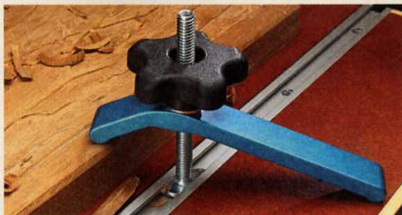
▲ Hold-Down Options. Shop-made hold-downs (top) or purchased ones (bottom) make it easy to clamp your workpiece securely.
