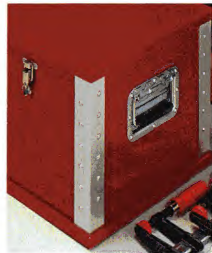
▲ Light & Strong. Riveting sections of aluminum angle into the corners make this one sturdy tool chest.
