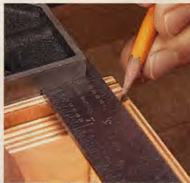
▲ Lay Out Corner. Use a pencil and a combination square to mark the layout lines to guide the chisel.
