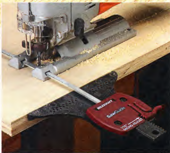
▲ Not Just an Edge Guide. The Milescraft SawGuide keeps your jig saw parallel to an edge while cutting straight lines (above) and also holds the line when cutting perfect circles (top).
