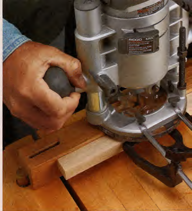
▲ Upcut Bit. The flutes of an upcut bit allow the bit to cut mortises fast with a plunge router.
