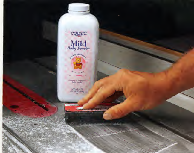
▲ Powder. Talc found in baby powder protects cast iron and creates a slick surface.
