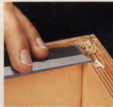
▲ Remove Waste. After defining the corner with a vertical cut, clean out the waste with a paring cut.
