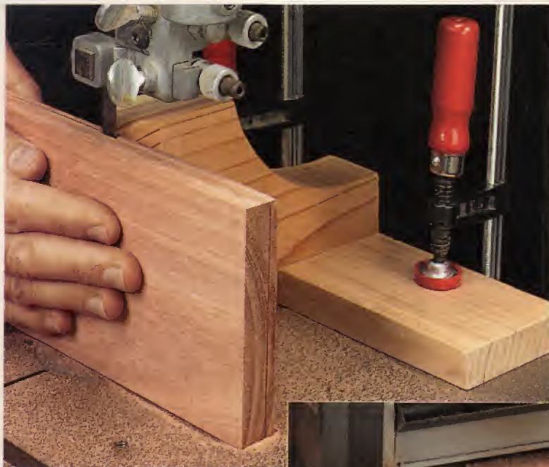
▲ Resawing. A simple pivot block helps you keep the blade cutting on the layout line.
