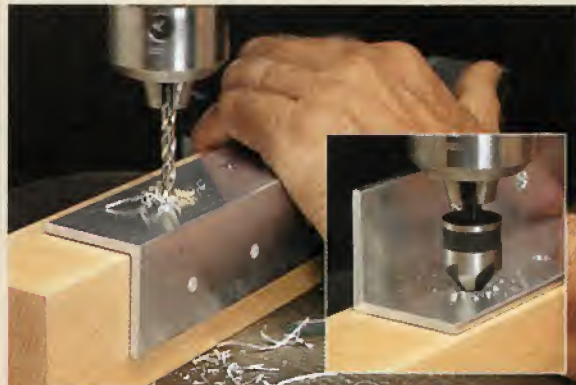
▲ Drill the Holes. Using a hardwood backer board for support, carefully drill the holes in each corner. Use a countersink to clean up the holes.
