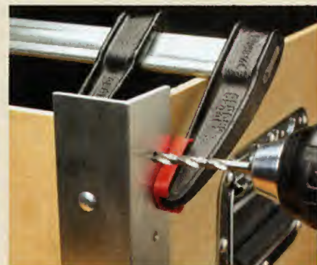
▲ Install Side Panels. After riveting the corners to the front and back panels follow the same procedure for the sides.
