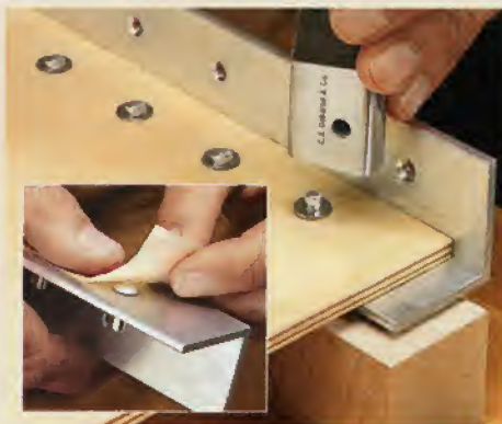
▲ Install Rivets. Tape rivets to hold them in the angles. A riveting tool "mushrooms" them for a secure connection.
