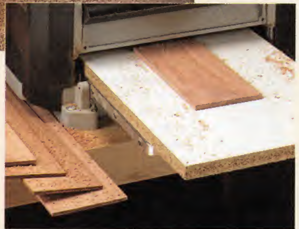
▲ Planing Sled. Each strip is fastened to a sled with double-sided tape for planing.
